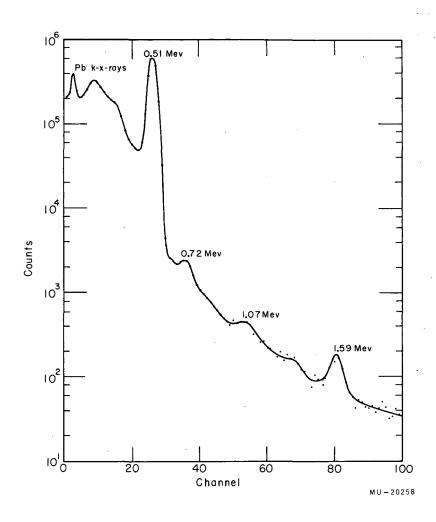
Fig. 2. Gamma-ray spectrum of Sm 142 -- Pm equilibrium mixture taken with a 1-1/2-inch by 1-inch NaI(T1) crystal. Beryllium absorbers were used above and below the sample to annihilate the positrons; a lead absorber was used to remove the K x-rays.
