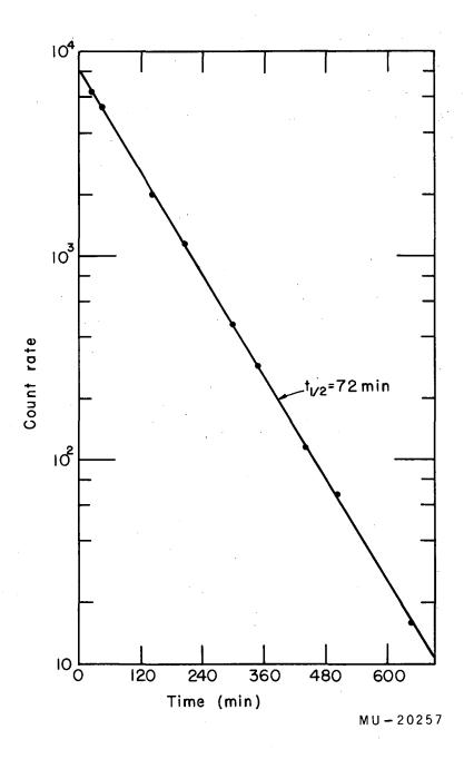
Fig. 1. Decay curve of the annihilation radiation of  ${\rm Sm}^{142}$  --  ${\rm Pm}^{142}$  equilibrium mixture.
