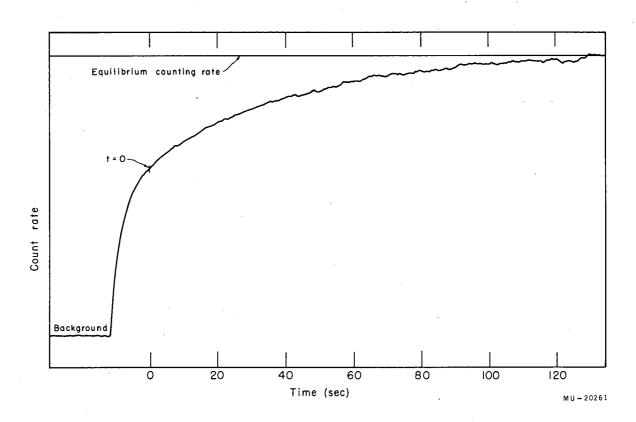
Fig. 5a. Growth curve of Pm 142 into Sm 142.
