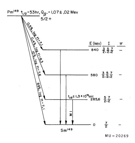
Fig. 12. Decay scheme of Pm 149.
