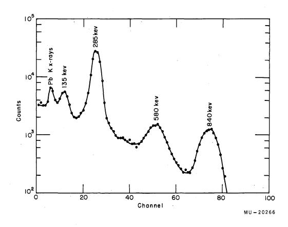
Fig. 9. Gamma-ray spectrum of Pm<sup>149</sup> taken with a 3-inch by 3-inch NaI(Tl) crystal and a 4 gm/cm<sup>2</sup> lead absorber.
