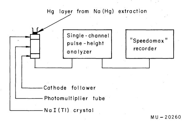
Fig. 4. A schematic diagram of the counting arrangement used in measuring the half-life of  $Pm^{142}$ .
