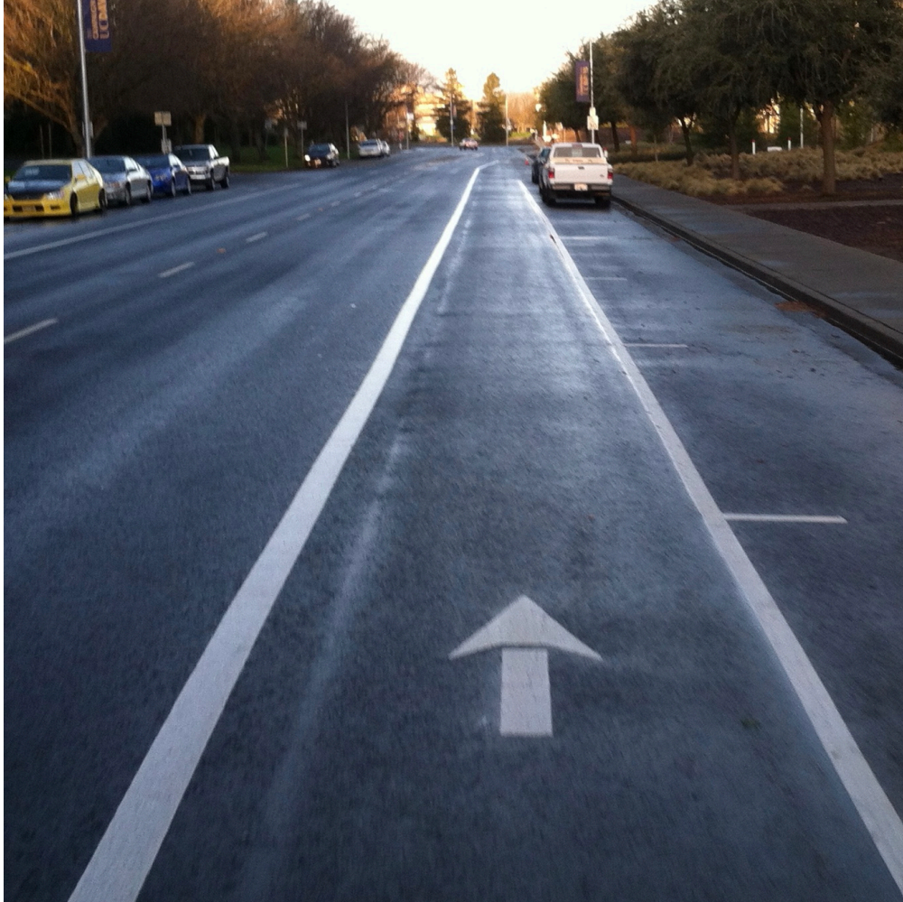
Figure 3. An example of a conventional bicycle lane
