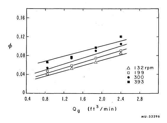
Fig. 20. Gas holdup vs superficial gas velocity; impeller A-1; isopropyl alcohol.
