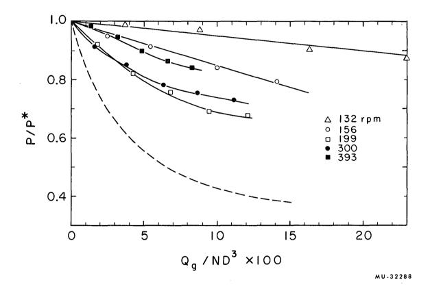
Fig. 12. Ratio of two-phase to single-phase power consumption, as function of ratio of gas flow to impeller flow; impeller A-4. --- Curve given by Hyman.
