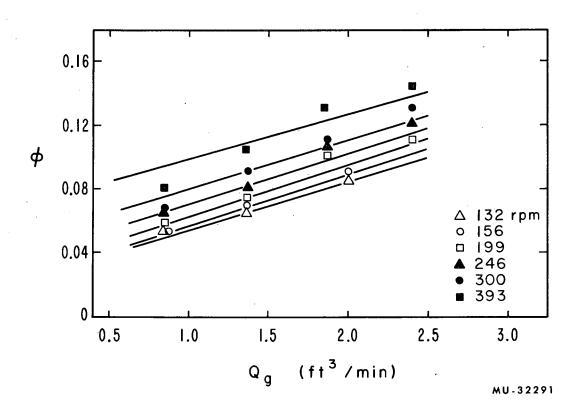
Fig. 15. Gas holdup vs superficial gas velocity; impeller A-1. Points from experimental data; curves calculated from correlation.
