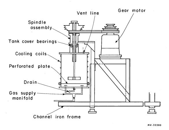
Fig. 1. Mixing vessel, drive assembly, and stand.
