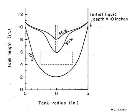
Fig. 6. Contours for volume fraction of air in baffled open-top vessel; impeller A-2, 393 rev/min.
