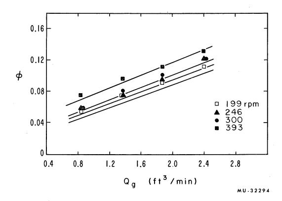
Fig. 18. Gas holdup vs superficial gas velocity; impeller A-5. Points from experimental data; curves calculated from correlation.
