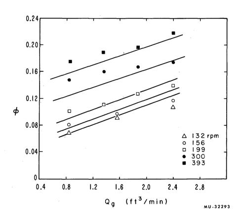
Fig. 17. Gas holdup vs superficial gas velocity; impeller A-4. Points from experimental data; curves calculated from correlation.
