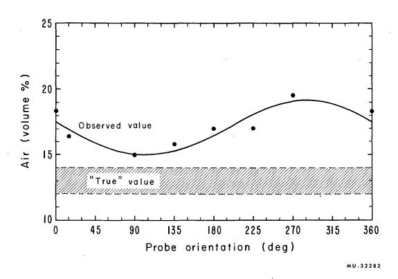
Fig. 5. Effect of probe orientation upon observed volume\_fraction of gas phase.
