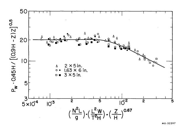
Fig. 4. Correlation of power number for various impeller sizes and positions.
