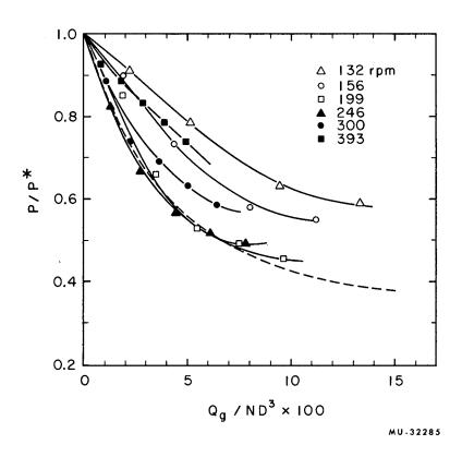
Fig. 9. Ratio of two-phase to single-phase power consumption, as function of ratio of gas flow to impeller flow; impeller A-3. --- Curve given by Hyman.
