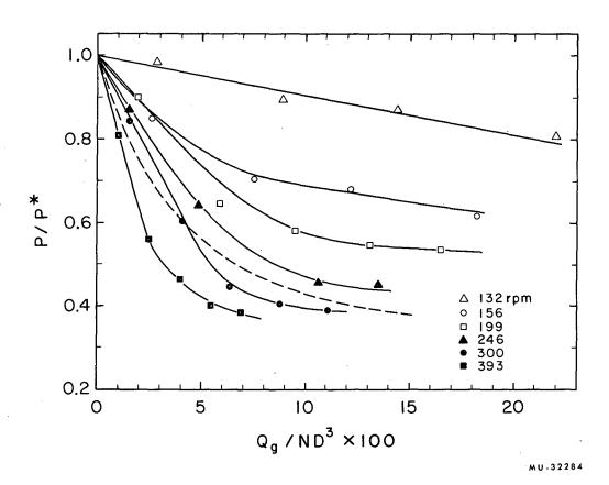
Fig. 8. Ratio of two-phase to single-phase power consumption, as function of ratio of gas flow to impeller flow; impeller A-1. --- Curve given by Hyman.
