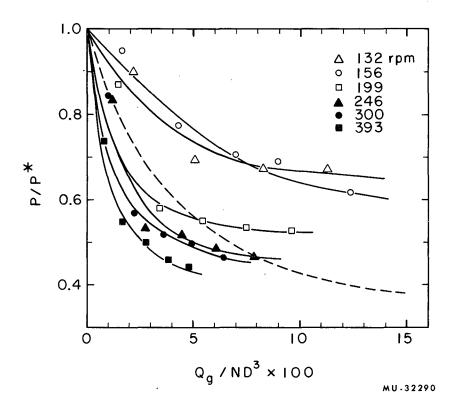
Fig. 14. Ratio of two-phase to single-phase power consumption, as function of ratio of gas flow to impeller flow; impeller B-1. --- Curve given by Hyman.
