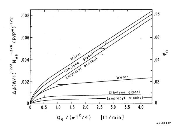
Fig. 11. Correlation of gas holdup based on gas flow, physical properties, and agitation conditions.
