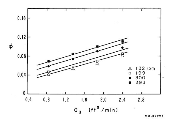
Fig. 19. Gas holdup vs superficial gas velocity; impeller A-1; ethylene glycol-water mixture.
