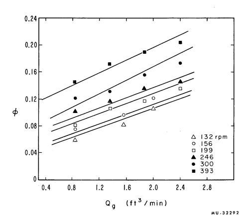
Fig. 16. Gas holdup vs superficial gas velocity; impeller A-3. Points from experimental data; curves calculated from correlation.
