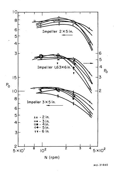
Fig. 3. Effect of speed on power number at different distances between bottom edge of impeller and bottom of vessel.
