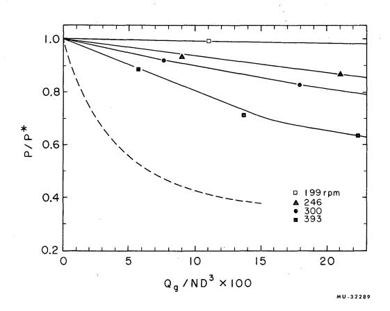
Fig. 13. Ratio of two-phase to single-phase power consumption, as function of ratio of gas flow to impeller flow; impeller A-5. --- Curve given by Hyman.
