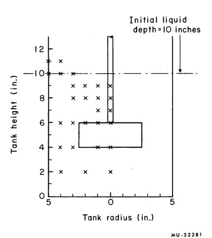
Fig. 2. Array of gas-liquid sampling points in mixing vessel.
