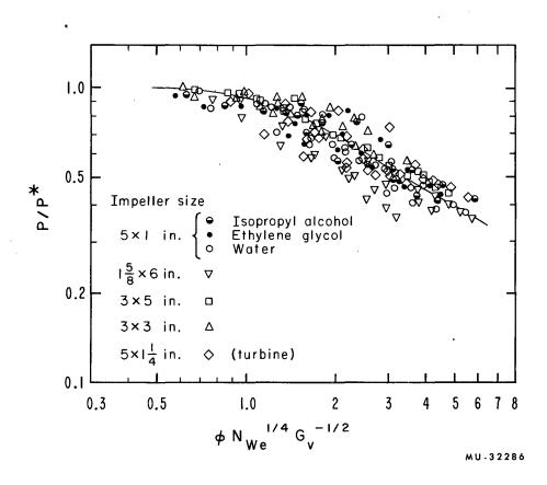
Fig. 10. Correlation of two-phase-to-single-phase power ratio, based on gas holdup, Weber number, and a geometrical factor.
