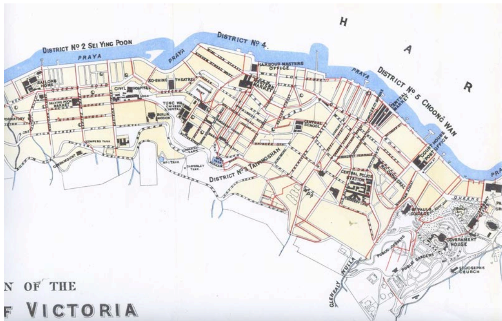
Figure 3.5. Plan of Victoria showing the layout of new water mains proposed by Chadwick. (Source: The National Archives of the U.K., Public Records Office, London).
