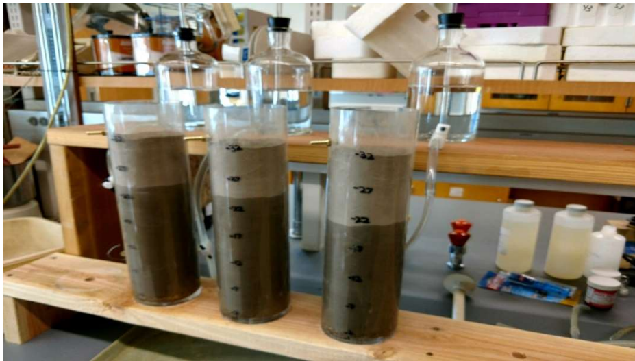
Figure 1. The soil columns were saturated by saline solution from the bottom to the top using Mariotte bottles to establish initial distribution of soil salinity for the leaching experiments.
