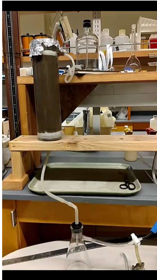
Figure 5. Illustration of a Mariote bottle applying water to clay soil under unsaturated conditions. The hydraulic head of the bottle is underneath the soil column demonstrating capillary flow. Vacuum matric suction of approximately 100 cm was applied underneath the columns to facilitate leachate collection for the clay soil.
