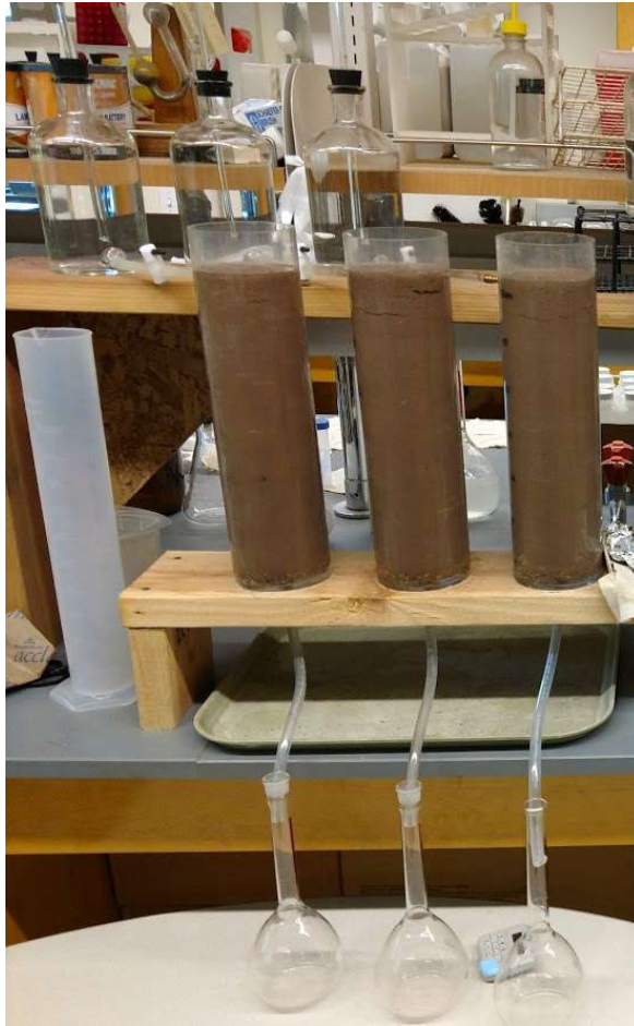
Figure 3. Illustration of the Mariotte bottles applying water to the soil columns at a constant head under gravimetric flow and collection of leachates from the drainage outlets. Ponding is present given saturated conditions. The water valve in the figure is used to turn the water application on and off for the intermittent treatment.
