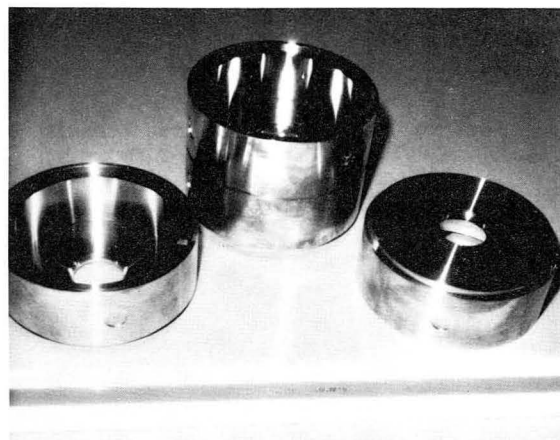
Figure 5. Components for a model of the ALS linac structure, fabricated and assembled at the Stanford Linear Accelerator Center. Precision milling of the cuplike components results in tolerances of a fraction of a mil.
