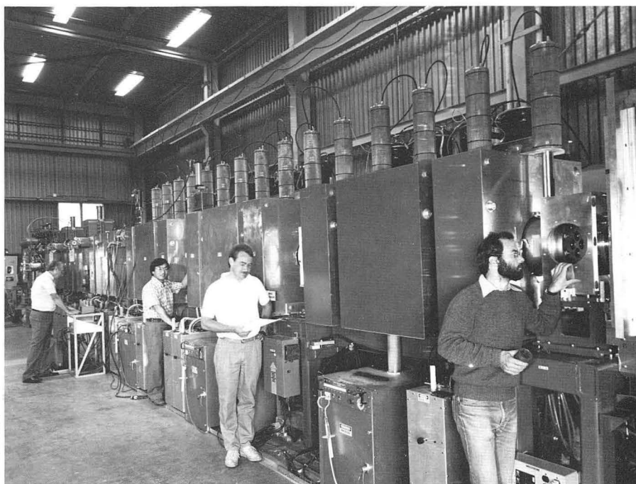
Figure 24. The completed apparatus for the multiple-beam experiment MBE-4. The injector is at the far end; the rectangular enclosures house the 24 accelerating cores.
