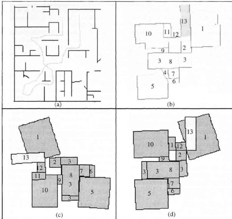
Figure 3.(a) The environment traversed, (b) a cognitive map computed from exact ASRs (c) the viewer's interpretation of a cognitive map computed from fuzzy ASRs where the viewer has no locational information for the exits. (d) the viewer's interpretation of a cognitive map constructed from fuzzy ASRs where the viewer knows on which side of the fuzzy ASR the exits are located but not their exact position.
