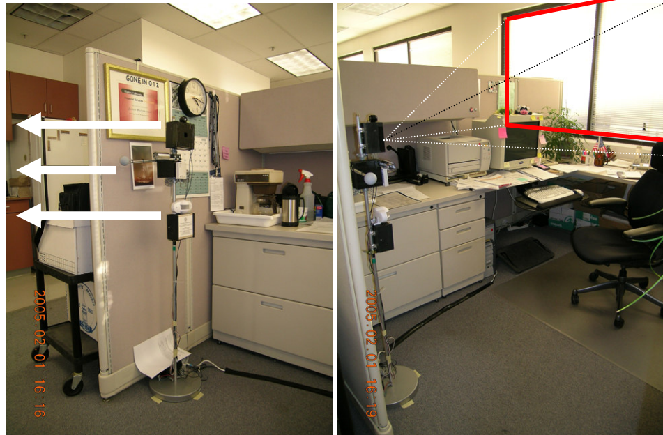
Figure 3.29 Pictures of the instruments in the field. The “lighting” box and the “temperature” box were attached to a free-standing pole at 4 ft (1.22m) and 3.6 ft (1.10m). The occupancy sensor was also mounted to the same pole. The opening of the “lighting” box was positioned to measure average window brightness (left)
