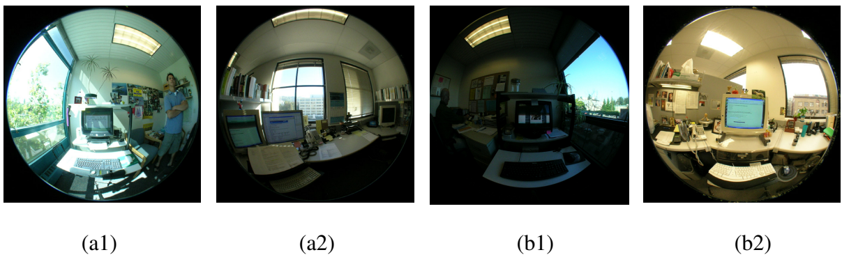
Figure 3.11 Direct solar penetration categories: a1) direct sun falling on occupants, a2) direct sun falling on the room surface but not on occupants, b1) no direct sun (clear sky), and b2) no direct sun (cloudy sky)
