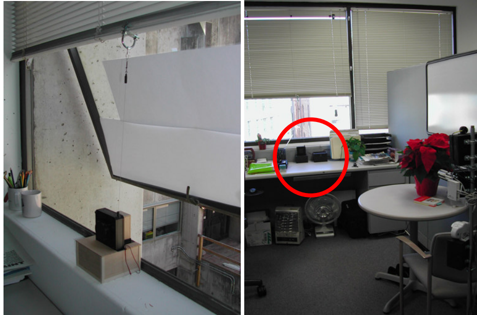
Figure 3.12 Installation of string potentiometer in the workspace. A common 1.5-inch U-bolt was attached to the bottom of the Venetian blind which created a connection point for the string potentiometer (left). The potentiometer unit was anchored to a wooden box, filled with a 4" x 4" concrete block. The potentiometer unit is portable and can be reused. The unit is painted black to blend with other office supplies (right).
