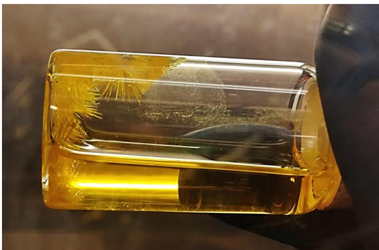
Figure 2.8. Crystals of (C_5Me_5)_2Dy(C_3H_5) grown using a square Nd_2Fe_{13}B magnet attached to the top side of the vial from which the mother liquor has been removed to demonstrate the external magnet elicits crystal growth on the wall with which it is in direct contact.
