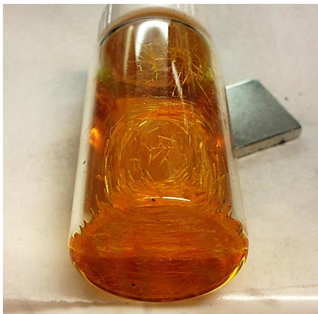
Figure 2.7. Crystals of (C_5Me_5)_2Tb(C_3H_5) grown using a square Nd_2Fe_{13}B magnet attached to the side, demonstrating this phenomenon can be generalized to many different paramagnetic species.
