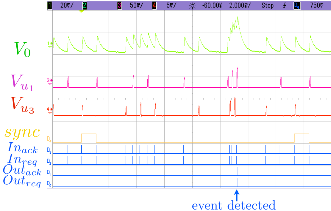
Figure 6.4: Oscilloscope traces showing periodic synaptic input train of excitatory synaptic events with constant synaptic conductance strength amplitude and varying delay between events resulting in neural event activation.
