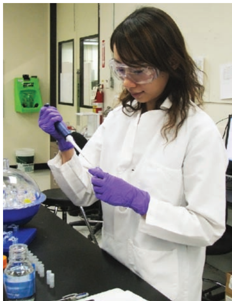
UC Riverside Ph.D. student Qing Qin uses a pipette to measure enzymatic hydrolysis samples into vials, in order to determine sugar concentrations. This research ultimately seeks more efficient ways to break down plant cellulose into sugars that can be fermented into transportation fuel.
