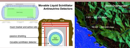
Modular and movable detectors with a volume of ~100 tons combined with an active muon veto allow a precision measurement of  $\theta_{13}$ . A variable baseline is critical for controlling systematics and demonstrating the subdominant oscillation effect associated with  $\theta_{13}$ .
