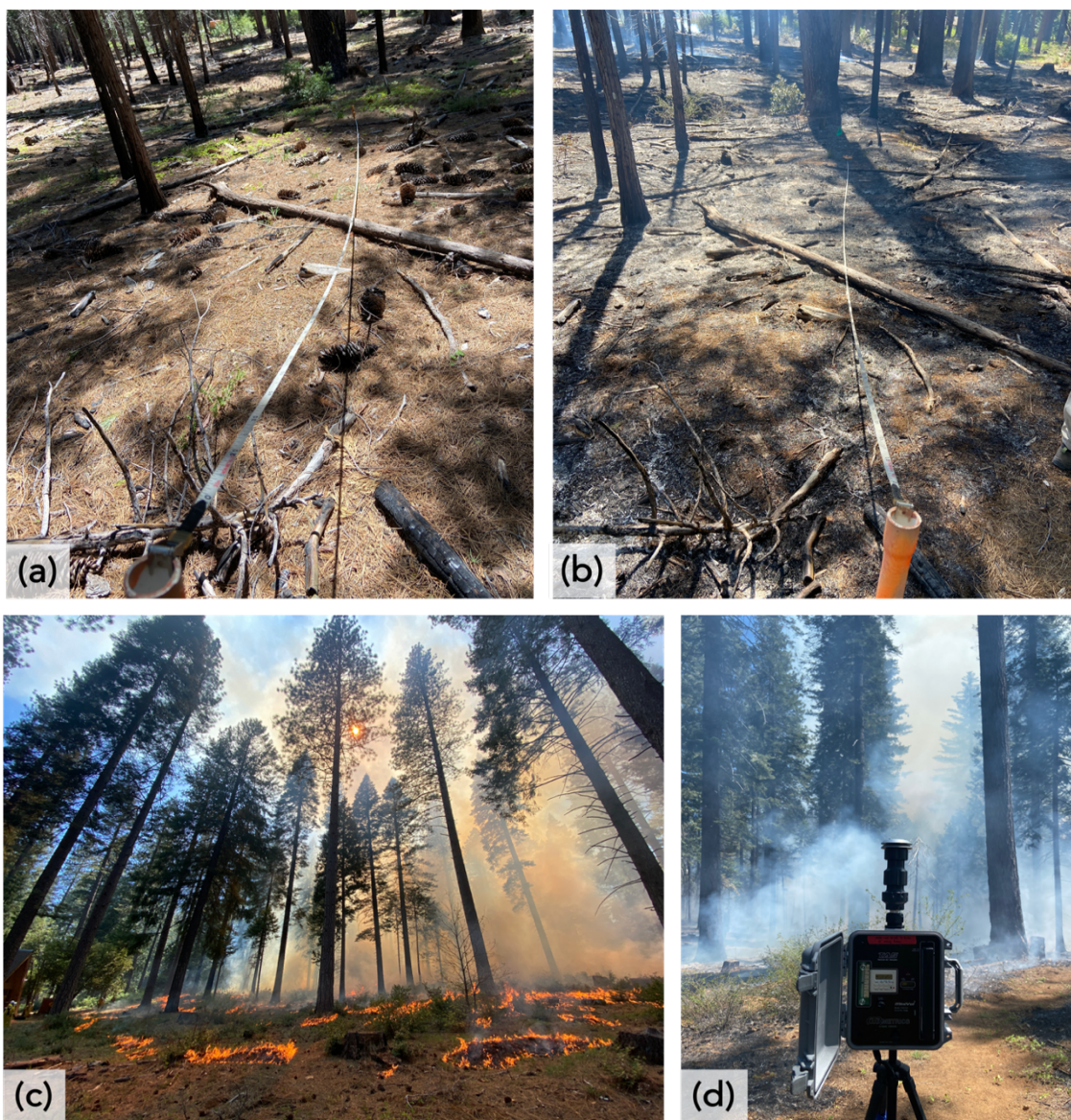
Figure 4.2. Photos taken at the Blodgett Forest Research Station during a prescribed fire in May 2022. Photos at the top show a transect (a) before and (b) after the fire (Plot 2). By comparing the before and after photos, it is evident that most of the pinecones and smaller-diameter dead fuels were consumed. Bottom photos show (c) active flaming in plot 14 of the unit on 14 May 2022 and the (d) AirMetrics Tactical Air Sampler with PM 2.5 impactor mounted on top (right), with a PurpleAir PA-II sensor secured to its back.
