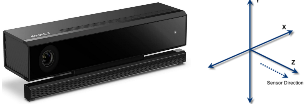
Figure 3: Microsoft Kinect V2 (left) and its coordinate system (right).
