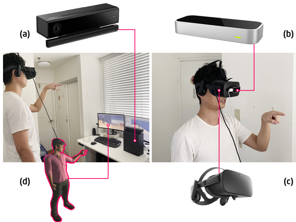
Figure 3.3: Device arrangement for VR interaction in GesTHOR. The human player wears an (c) Oculus headset with (b) LMC. (a) Kinect is placed 1.5m from the human player and 1.5m above the ground. The screen displays (d) A humanoid agent that are mirroring the body and hand movements.
