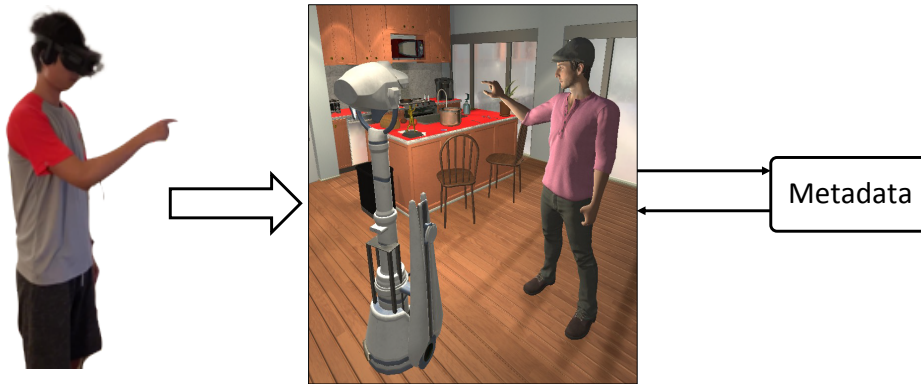
Figure 3.6: Replay a recorded program. Users can always replay the recorded program in Unity, including scenes, objects, and human motions.
