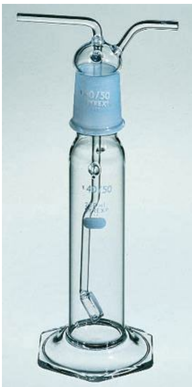
Figure 4.3 Example of liquid vapor separator with a Pyrex glass bubbler.
