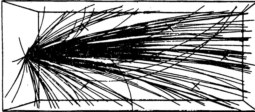
Fig. 6. Schematic of the reconstruction of a 960 MeV/nucleon U + U central event in the LBL streamer chamber. The event was measured by the UC Riverside group and contains over 100 charged tracks.
