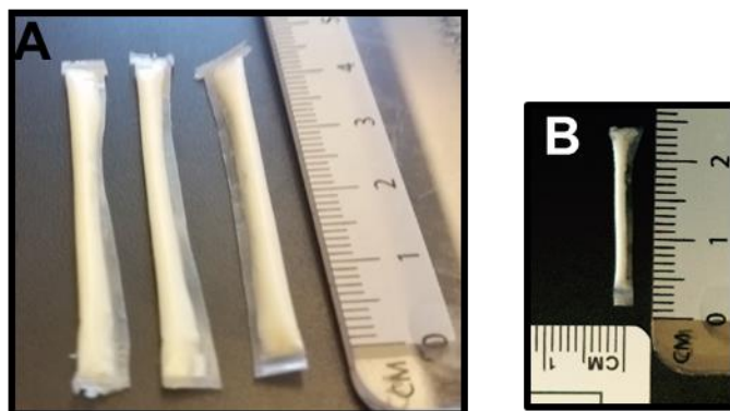
Figure 54 TAF TFPD Prototypes. (A) 2.5mm diameter, 40mm long prototypes loaded with 230mg 1:1 TAF:PEG300 (w/w). (B) 0.6mm diameter, 20mm long prototype loaded with 26mg 1:1 TAF:PEG300 (w/w).
