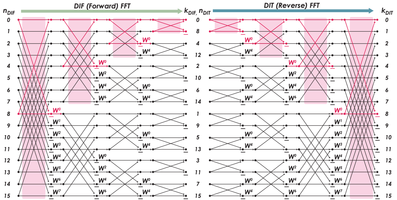
Figure 2.1: N = 16 , radix-2 DIF (a) and DIT (b) CTA signal-flow graphs [34]. One butterfly “group” (containing N/2^i butterflies for the DIF FFT) in each of the four N/2^{i-1} , i \in [1, 4] decomposition stages is highlighted. The number of butterfly groups in the i th stage is given by 2^{i-1} . Different butterfly groups within the same stage share the same twiddle factors. Example radix-2 DFT butterflies are in pink.
