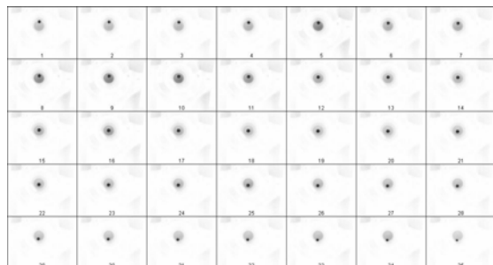
Figure 6: Electron beam deflection height through a 2 cm scintillator. Dark center spot is an e-beam spot deflected from up to down as shown by numerical numbers.
