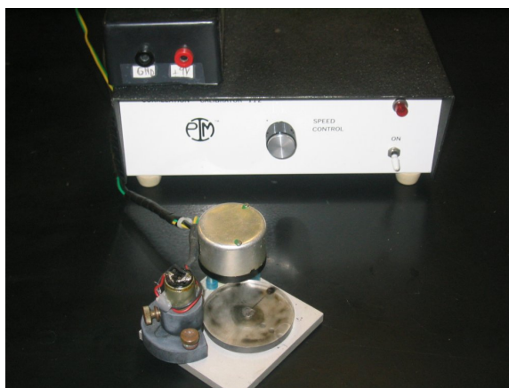
Figure 2.31: Picture of the spinning disk setup used to validate the Image Pro tracking of fluorescent blood cells. Fluorescent microspheres were placed on the surface of the plastic disk which spins at a constant rate determined by the potentiometer setting. A single revolution was timed and recorded simultaneously. With the distance from the center to the optical viewing location, the linear velocity may be calculated. The calculated linear velocity is then compared to the output from the Image Pro tracking module.
