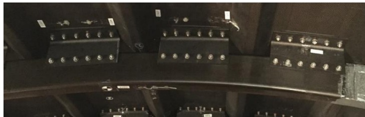
(a) Full assembly with C-frame and shear ties
