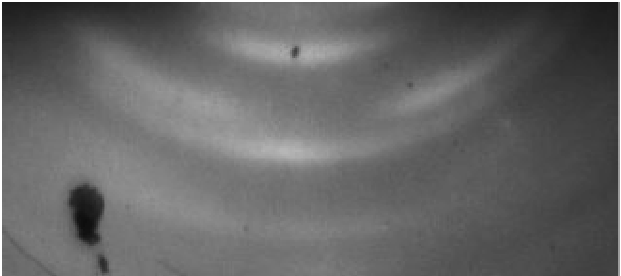
Figure 2.4: RHEED diffraction pattern for polycrystalline MgO grown onto amorphous \text{Si}_x\text{N}_{(1-x)} .
