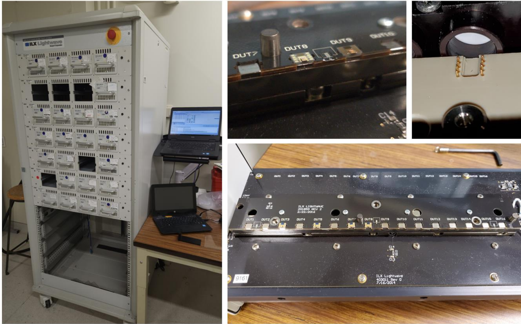
Figure 2.8. (Left) Overview of aging rack system with 7 shelves with up to 4 fixtures per shelf. (Bottom right) View of an opened fixture with 16 slots for laser carriers. The fixture head with spring-loaded contact pins and photodiodes (pictured in top right) is placed on top of this. (Top middle) Magnified view of carriers in testing slots next to a fixture head alignment pin.
