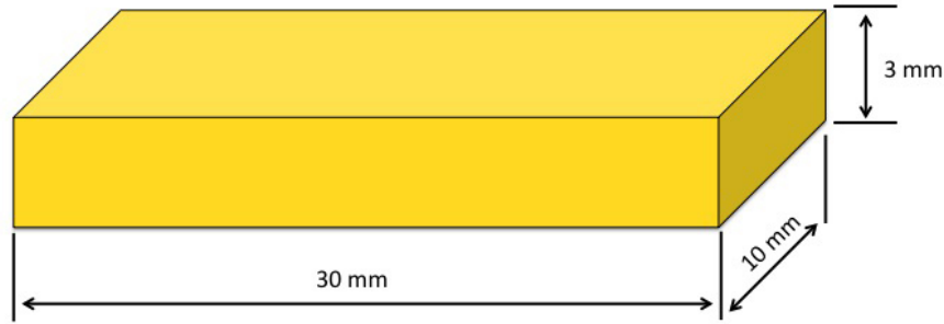
Figure 3.19: Dimension of the sample for single cantilever test
