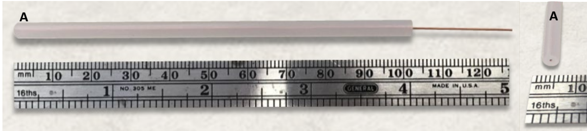
Figure 6.1 Wire sample type A used in combined forced flow, sub-atmospheric ambient pressure, and elevated oxygen concentration study.
