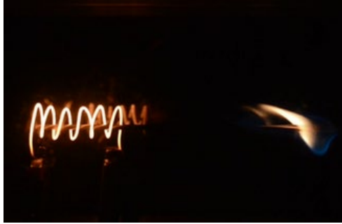
Figure 4.4 Ignition Method III – igniter remains on until the flame spreads along entire wire length.
