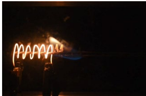
Figure 4.3 Ignition Method II – igniter turned off when the flame spreads past igniter coils.
