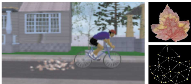
5 The leaves are influenced by wind fields generated by moving objects such as a bicyclist. The diagram on the right shows the texture map and the spring and mass network used to model a leaf. For clarity, additional springs that resist bending and shear aren't shown.
