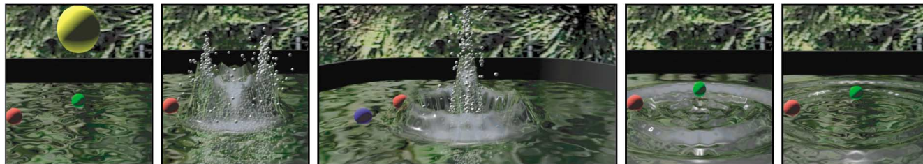
10 Two-way coupling is used to model the interaction between floating balls and water in a small pond. When the lighter balls are dropped into the water, they create small disturbances and float on the surface. The larger, denser ball creates a larger disturbance and sinks. The resulting waves affect motions of the floating balls.
