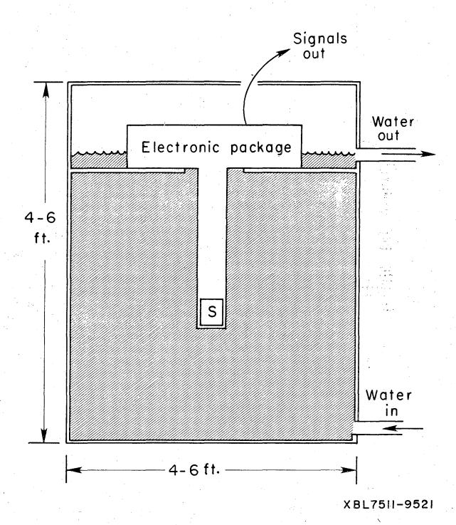
Fig. 2. Schematic layout of field facility for Rn-222 measurement in water by  $\gamma$ -ray spectrometry.
