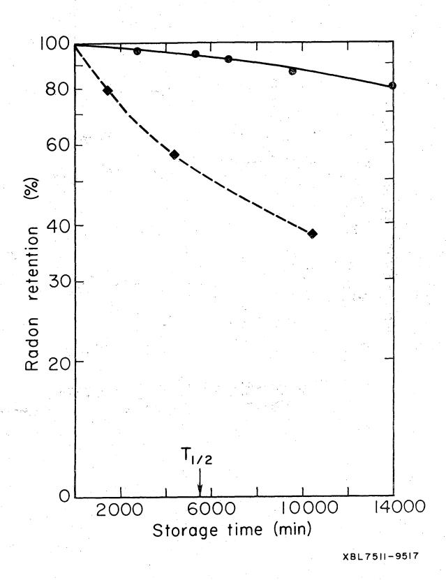
Fig. 4. Retention of Rn-222 in water for two types of polyethylene sampling containers.
