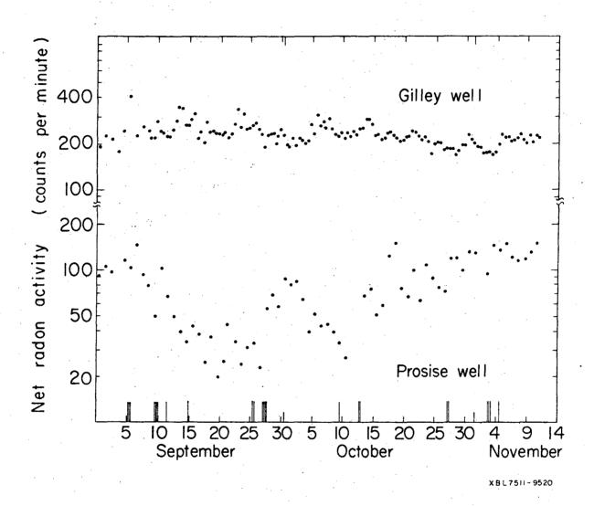
Fig. 5. Results of Rn-222 measurements in the discrete sampling program from two bedrock wells in the Oroville area.
