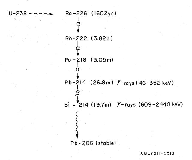
Fig. 1. Partial decay scheme of the U-238 series.
