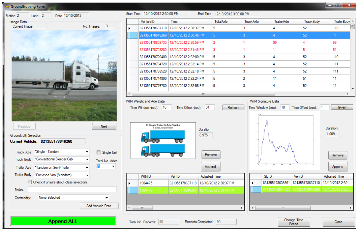
1 2 Figure 3 Integrated Data System User Interface Example for Vehicle Classification
