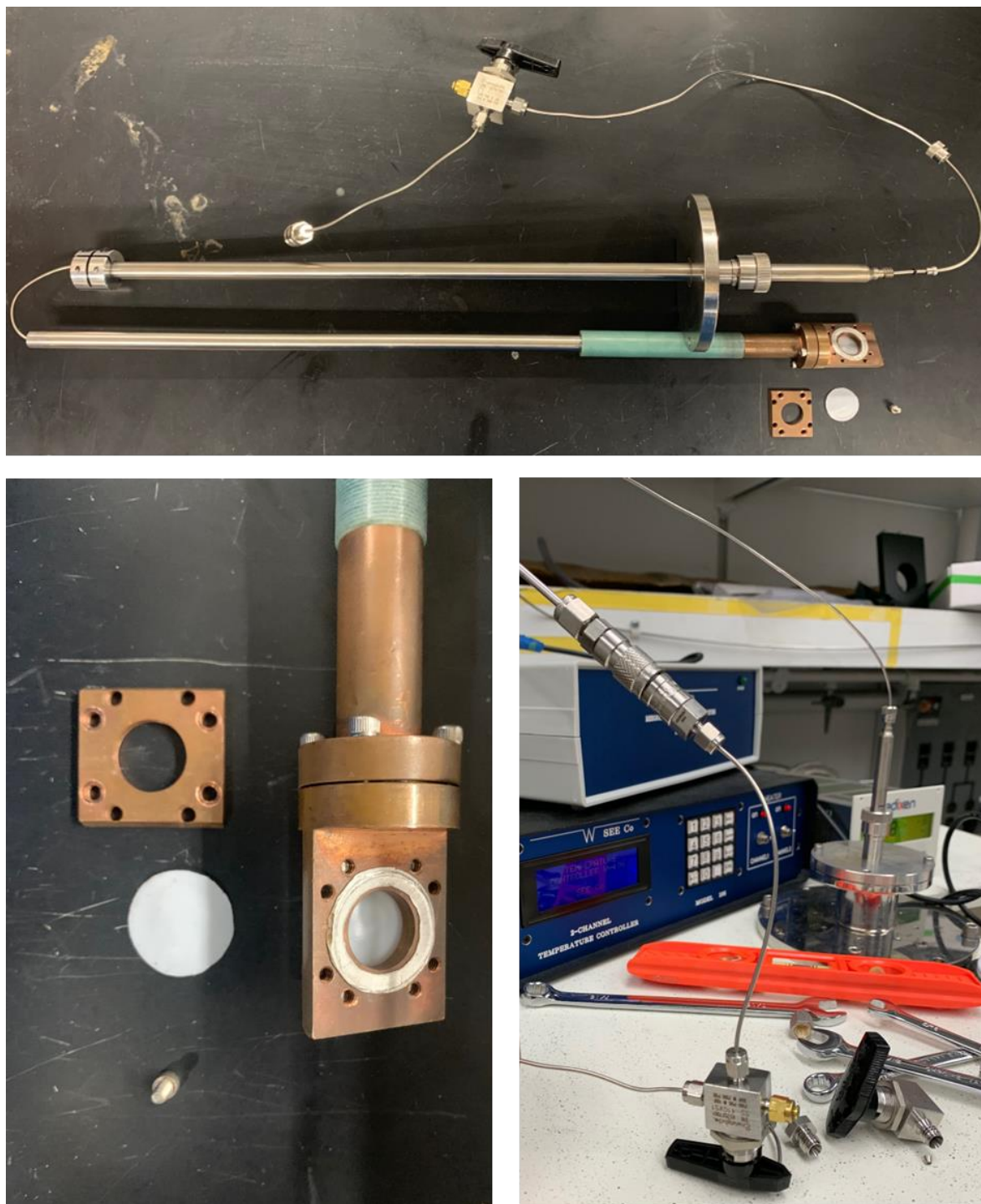
Figure 2.S25. Disassembled in situ gas dosing cell (top), closeup of the copper sample holder with Teflon window and indium gasket shown after compression (bottom left), gas line connections and insertion into the instrument (bottom right).
