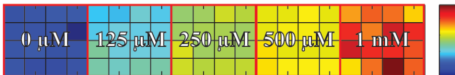
Figure 4.6. Heat map of measured data from the entire 16-sensor array with different redox molecule concentrations applied.
