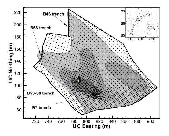
Figure 14. Boundary and the plan view of the three-dimensional mesh for the refined model, with four trenches implemented for restoration. The background is the measured concentration contour with the contour legend shown in Figure 13. The right upper-corner plot shows a close-up view of the sump and the B7 trench system for controlling the contaminant source.
