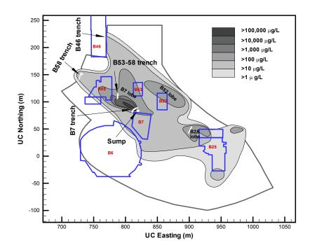
Figure 2. Contaminant plumes observed at the LBNL's Old Town site in 2003 (gray flood) and groundwater collection trenches (white polygons) installed for restoration.
