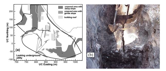
Figure 6. (a) Three different types of infiltration areas in addition to the default paved area, and three detected leaking storm drains and other underground utilities. (b) Evidence of ruptured concrete pipes observed in the field.
