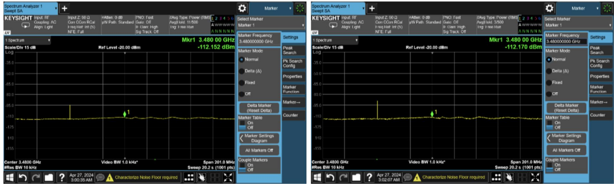
Fig 4.4.9 (a) RF input power at 0 dBm (b) RF input power at 10 dBm
