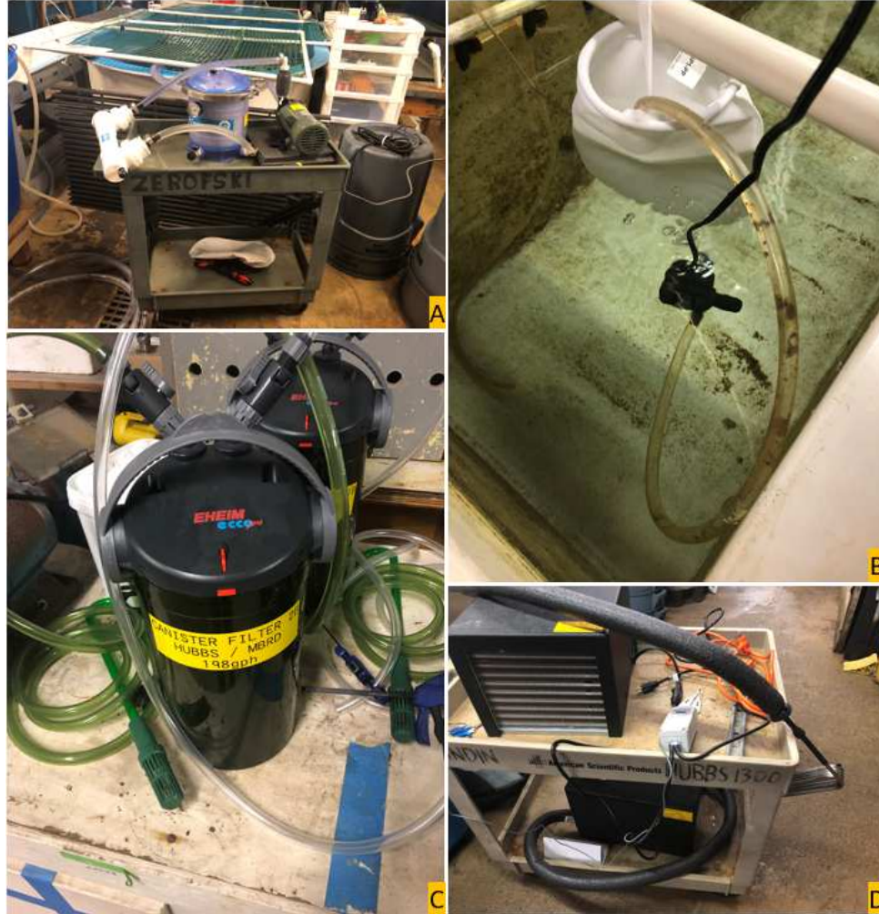
Figure 10: Crash carts and emergency maintenance equipment. (A) Water pump connected to both a canister filter and UV sterilizer. (B) Emergency filter setup with small powerhead flowing water through a filter bag. (C) Canister filter. (D) Water cooler with arm to be submerged in tank.
