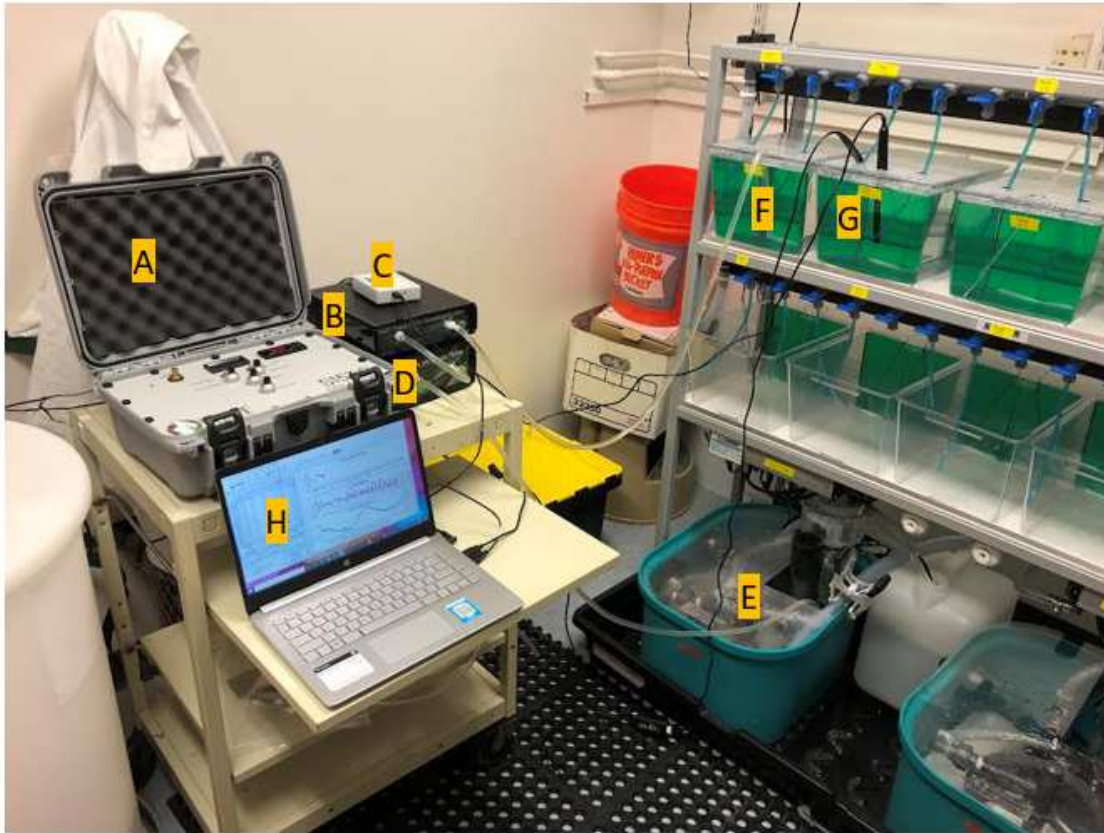
Figure 13: The Qubit Systems Rapid Dissolved CO 2 System set up and connected to both the coral RAS system and laptop with Logger Pro software. (A) S157-P CO 2 analyzer. (B) S400 DCO 2 Sampler. (C) LabQuest Mini data interface. (D) PL175 water pump. (E) Water intake line. (F) Water output line. (G) Salinity and temperature probes. (H) Laptop with Logger Pro software.
