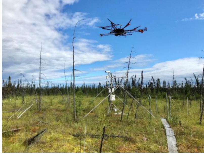
Figure 3.27: The mobile sUAS measurement platform above an eddy covariance tower in an Alaskan peatland bog.
