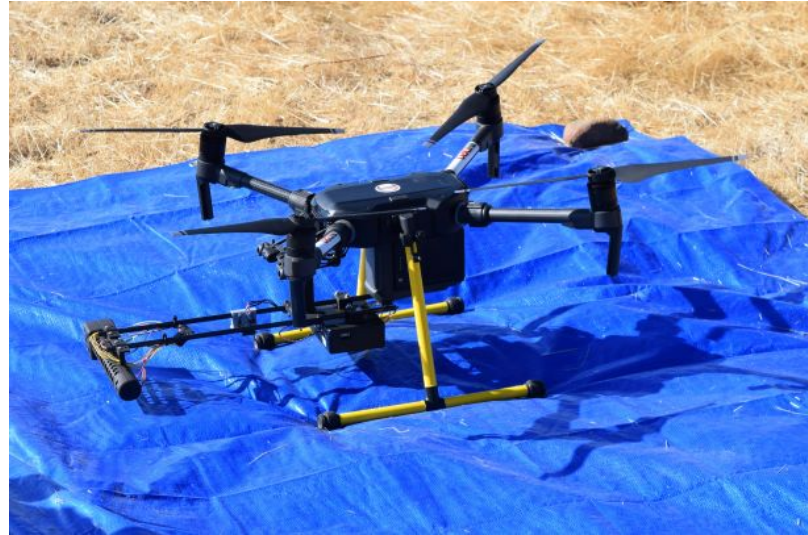
Figure 3.21: DJI Matrice 210 (M210) equipped with a sensitive methane sniffer developed by [9] and attached to the DJI Skyport.
