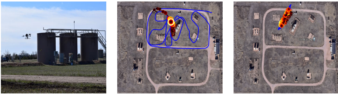
Figure 4.7: (a) Site level emission survey and quantification from METEC using TDLAS equipped drone. (b) The survey begins with a perimeter flight to identify leaking equipment. (c) Once a leak is identified the quantification can be done using downwind and upwind mass balance flights.
