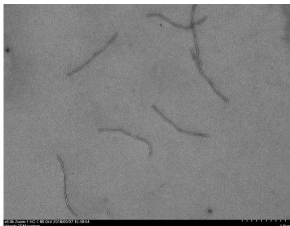
Figure 3.4. Transmission Electron Microscopy (TEM) Image of DNA Origami 10HB 5-mer Nanowires
