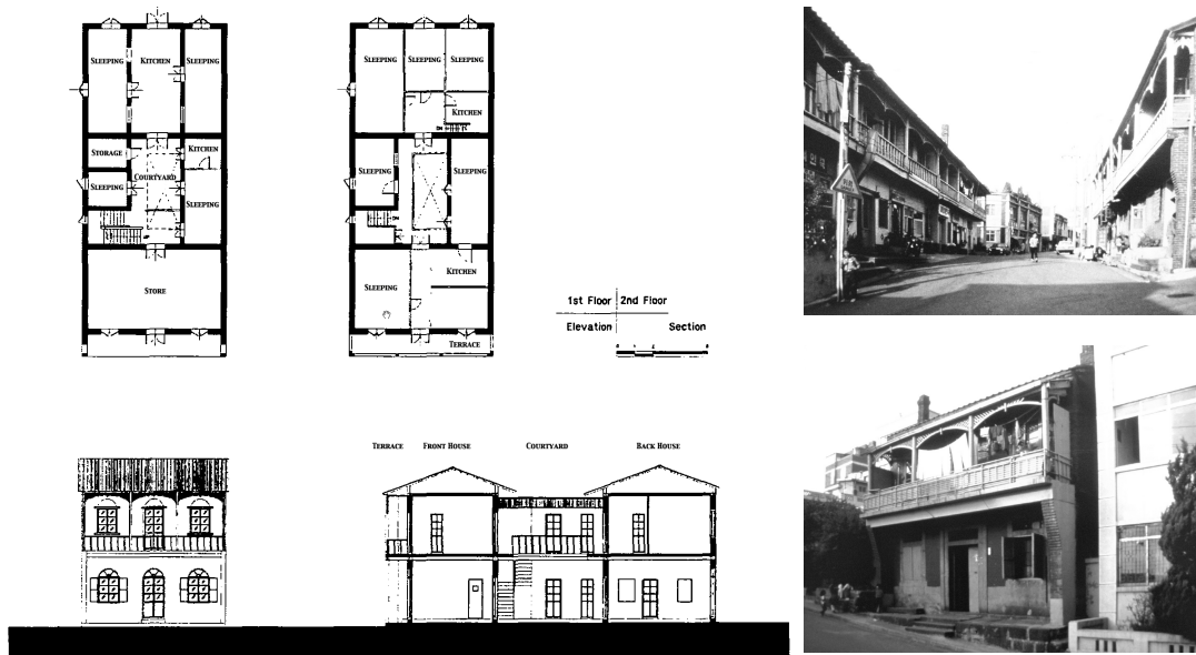
Figure 1-12. A typical example of shophouse in Incheon's Chinese settlement. Some of the shophouses built in the early twentieth century had remained until the 1980s, converted into lodging houses (Image Source: Chae 2003, left; Sonh Jang-won, right)
