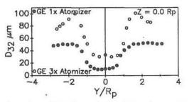
Fig. 2 Comparison of  $D_{32}$  between atomizers in the absence of the swirl cup assemblies
