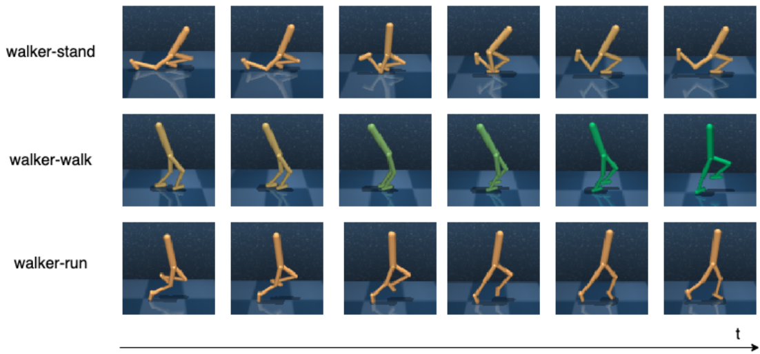
Figure 4.2: MuJoCo environment. Examples of three tasks (stand, walk and run) of MuJoCo walker robot. The agent has unique behavior in each task.
