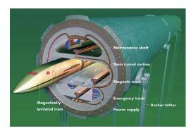
Researchers at MIT designed a vacuum-tube train system for a 45-minute trip from New York City to Boston in the early **1990s**. Like Musk's plan, the design called for a magnetic track.
