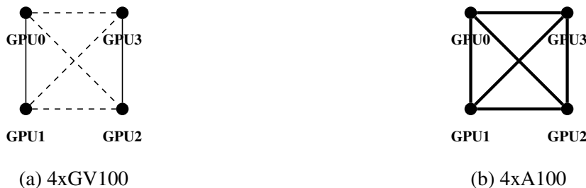
Figure 5.8: Communication topologies of the two multi-GPU platforms used in our experiments. Thin lines: 4 NVLinks (NV4); thick lines: 12 NVLinks (NV12); dashed lines: PCIe.
