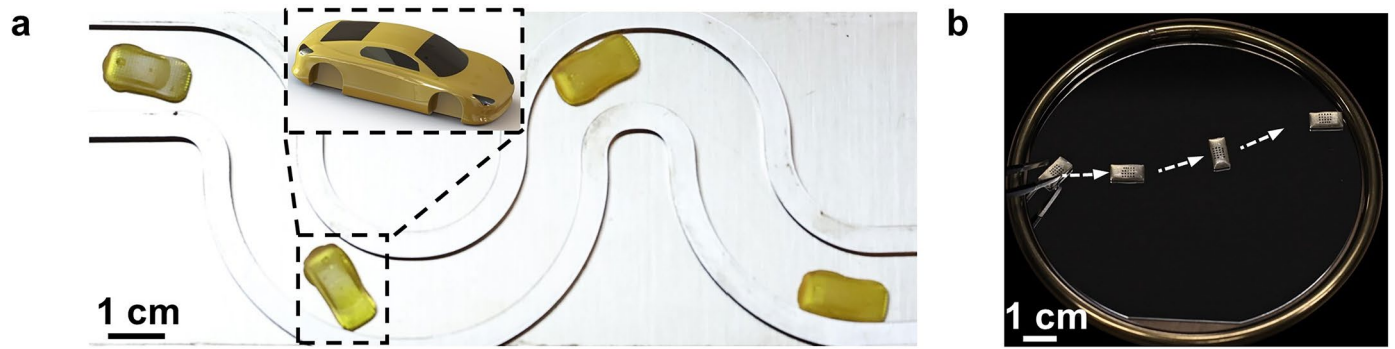
Extended Data Fig. 8 | Novel CS design attempts. a, Self-propulsion of a racing car prototype with tilted capillaries design on a horizontal track. The time interval between two consecutive frames is 1 second. b, Frictionless motion of metallic CS. The time interval between two consecutive frames is 0.5 seconds, and the T_{\text{sub}} is 280 °C.
