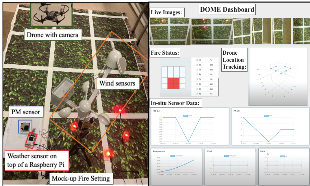
Figure 6.14: Sensors, Testbed and Dashboard in DOME
