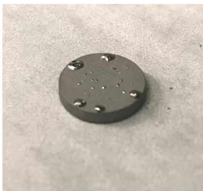
Figure 7: Image of Phase Separation on the Unpolished Surface of 90/10 Sample Sintered at 1250°C for 5 hours
