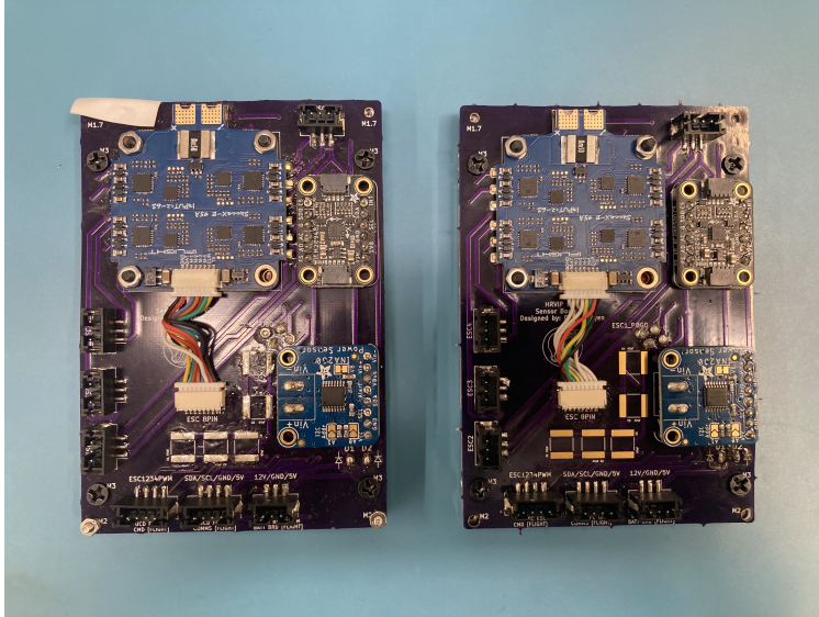
Figure 5.1: UC Davis / NASA JSC CubeSat HDD-RW PCB attached to back of HDD - Flight Unit and Engineering Unit
