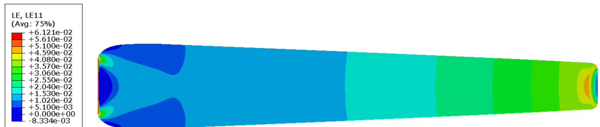
Fig. 6. Heatmap of strain distribution in the optic nerve (sagittal cross section; distal (closer to the eye) end to the left of the image, proximal (closer to the brain) end to the right), measured as a unitless ratio of tissue length after and before insult. “LE11” represents strain along the radial, i.e., transversal, direction. Warmer colors (positive values) indicate tensile strain, whereas cooler colors (negative values) indicate compressive strain.
