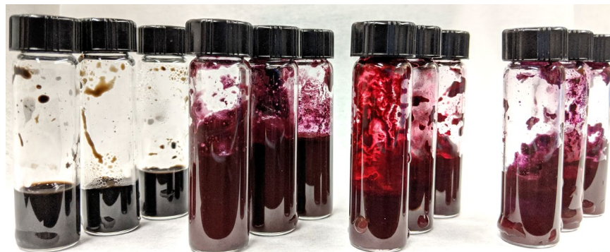
Figure 3.4 Reaction vials of standard graphene oxide suspension and PAB+GO suspensions. Far left: Standard GO suspensions. Right three: Varying mass ratios of PAB added to GO suspensions. Vials are 15 mm in diameter.
