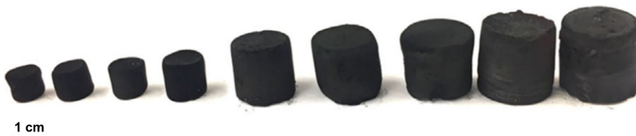
Figure 2.2 Graphene aerogels of varying sizes, from ~0.7 cm to 2.7 cm. Image credit to Dr. Sally Turner. 35
